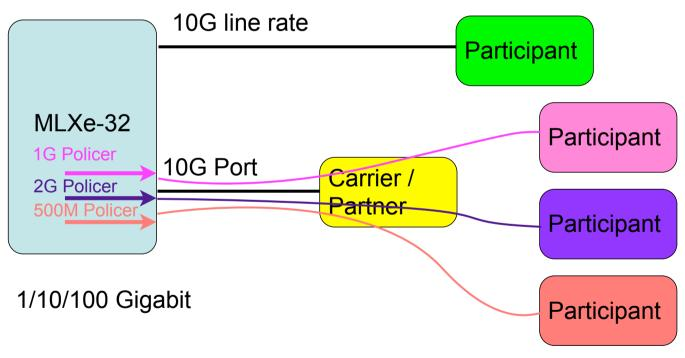
virtual and logical ports end up in the same VPLS instance - directly layer 2 connected
